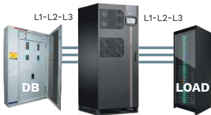
3-wire (L1-L2-L3) installation
